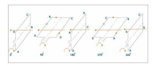
Such a current which changes its direction after equal intervals of time is called alternating current (AC).
