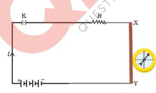
The needle is deflected which means that the electric current through the copper wire has produced a magnetic effect.
