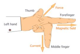
According to Fleming's left hand rule, when the thumb, forefinger and middle finger of the left hand are held mutually perpendicular to each other, with the forefinger pointing in the direction of the magnetic field and the middle finger in the direction of the current, then, the thumb points in the direction of the force exerted on the conductor.
