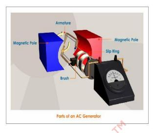
Armature is a soft iron core on which a coil having a large number of turns of insulated copper wire is wound. Magnetic poles are concave and cylindrical. The concave poles produce a radial magnetic field.
