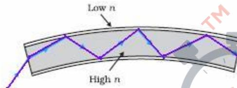
Light incident on one end of optical fiber at a small angle passes inside and undergoes repeated total internal reflections inside the fibre. It finally comes out of the other end, even if the fibre is bent or twisted in any form. There is no loss of light through the sides of the fibre. The only condition is that angle of incidence of light must be greater than the critical angle for the fibre material.
