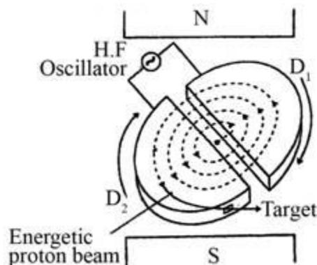
**Construction:** The construction of a simple cyclotron is shown in figure above. It consists of two semi-cylindrical boxes  $D_1$  and  $D_2$ , which are called dees. They are enclosed in an evacuated chamber. The chamber is kept between the poles of a powerful magnet so that uniform magnetic field acts perpendicular to the plane of the dees. An alternating voltage is applied in the gap between the two dees by the help of a high frequency oscillator. The electric field is zero inside the dees
