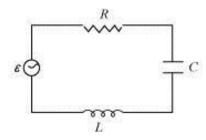
An ac source *E* having a voltage of  $v = v_m \sin \omega t$  is applied across the given LCR circuit.
