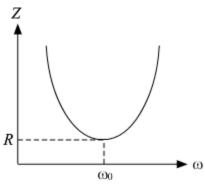
Here,  $\omega_0$  represents the resonance frequency for the LCR circuit and R is the resistance of the circuit.
