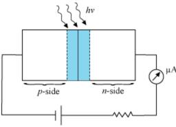
When visible light of energy ( $hv > E_g$ ) enters its depletion region, the electron-hole pairs are generated. These charge carriers are separated by the junction's electric field and are made to flow across the junction and cause reverse saturation current.
