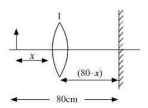
let object distance, u = x image distance, v = 80 - x focal length = f According to the lens formula:  $\frac{1}{f} = \frac{1}{v} - \frac{1}{u}$
