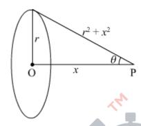
We need to find the electric field due to this charged ring at a point on the axis of the ring at a distance x from its centre.
