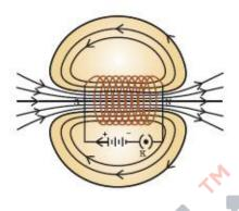
The field lines inside the solenoid are in the form of parallel straight lines. This indicates that the magnetic field is the same at all points inside the solenoid. That is, the field is uniform inside the solenoid.
