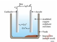
In electrolytic refining of copper, electrolyte is a solution of acidified copper sulphate. Anode is made up of impure copper. Cathode is made up of a strip of pure copper metal.
