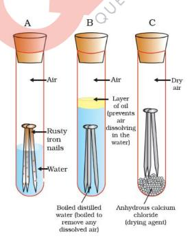
Conclusion: Both air and moisture are necessary for rusting of iron.
