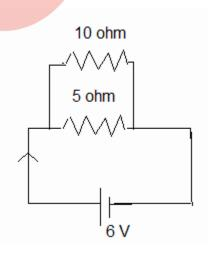
Total resistance in the circuit =  $(5 \times 10) / (5 + 10) = 50 / 15 = 10 / 3$  ohm Current in the circuit I =  $6 \times 3 / 10 = 1.8$  A
