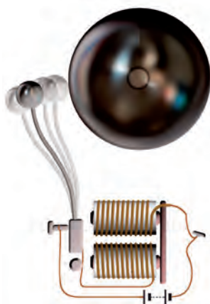
Fig. 14.20 Circuit of an electric bell
