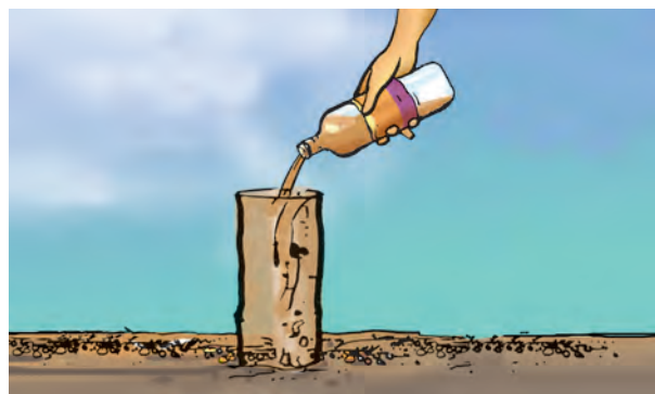
Fig. 9.5 Measuring rate of percolation
