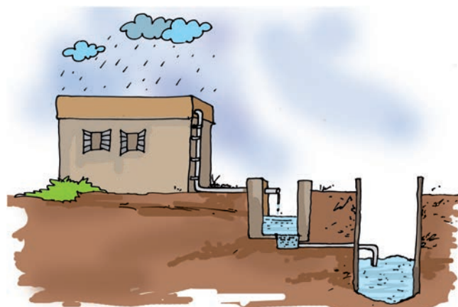
Fig. 14.13 Rooftop rainwater harvesting
