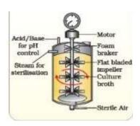
(c) The stirrer facilitates even mixing and oxygen availability throughout simple-stirred tank bioreactor, whereas in case of sparged stirred tank bioreactor, air is bubbled throughout the reactor for proper mixing.
