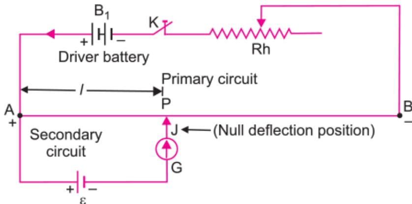
In primary circuit the rheostat (Rh) is so adjusted that the deflection in galvanometer is on one side when jockey is touched on wire at point A and on the other side when jockey is touched on wire at point B.
