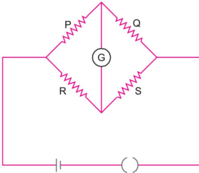
Working of a meter bridge is based on the principle of balanced Wheatstone bridge.
