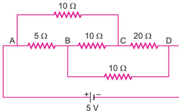
**Ans.** The equivalent wheat stone bridge for the given combination is shown in figure alongside.
