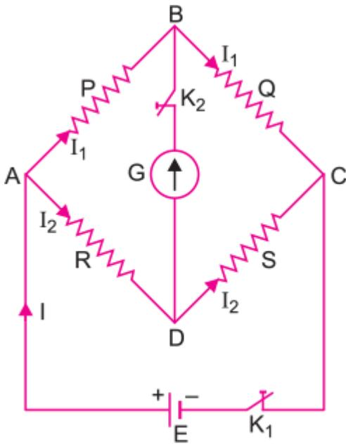
P, Q, R and S are four resistance forming a closed bridge, called Wheatstone bridge. A battery is connected across A and C, while a galvanometer is connected between B and D. When the bridge is balanced, there is no current in galvanometer.
