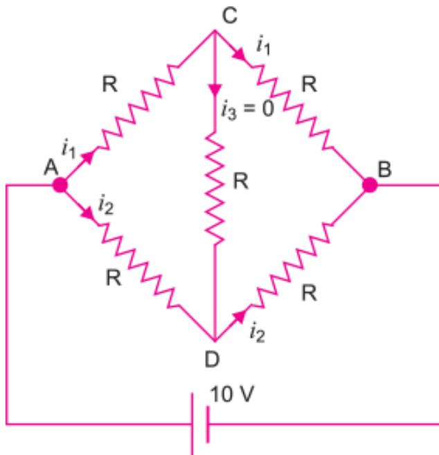
(i) The equivalent circuit is shown in fig. It is a balanced Wheatstone bridge. So, the resistance connected between C and D is ineffective.
