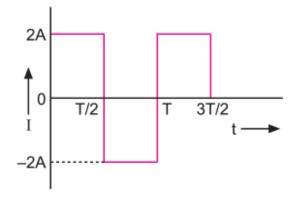
$$(I^2)_{\text{mean}} = \frac{\int_0^T I^2 \, dt}{\int \, dt} = \frac{\int_0^{T/2} (2)^2 \, dt + \int_{T/2}^T (-2)^2 \, dt}{T} = \frac{\int_0^T 4 \, dt}{T} = 4$$
