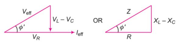
Phase angle,  $\tan \varphi = \frac{X_L - X_C}{R}$   $X_L = \omega \ L = 1000 \times 100 \times 10^{-3} = 100 \text{ ohm}$   $X_C = \frac{1}{\omega C} = \frac{1}{1000 \times 2 \times 10^{-6}} = \frac{1000}{2} = 500 \text{ ohm}$  $\therefore \qquad \tan \varphi' = \frac{500 - 100}{400} = 1 \quad \Rightarrow \quad \varphi' = 45^o$
