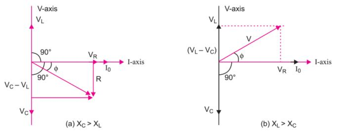
(ii) When  $X_L > X_C$ ; the phasor diagram is shown in fig. (b).
