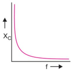
**Ans. Capacitive Reactance:** The opposition offered by a capacitor alone to the flow of alternating current through it is called the capacitive reactance.
