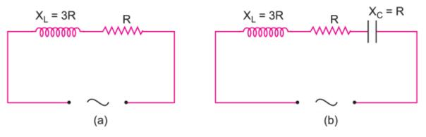
Impedance of circuit  $B_{*}Z_{B} = \sqrt{R^{2} + (X_{L} - X_{C})^{2}}$
