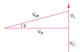
Q. 10. (i) Find the value of the phase difference between the current and the voltage in the series LCR circuit shown below. Which one leads in phase: current or voltage?
