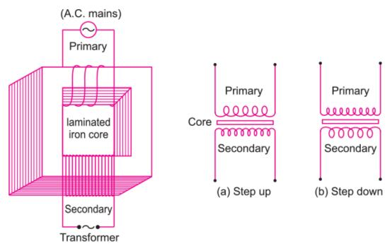
**Working:** When alternating current source is connected to the ends of primary coil, the current changes continuously in the primary coil; due to which the magnetic flux linked with the secondary coil changes continuously, therefore the alternating emf of same frequency is developed across the secondary.
