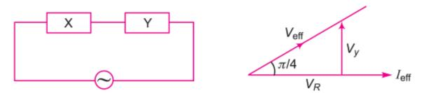
The voltage drop across the combination X and Y is ahead of the current flow. Hence, the element Y is an inductor.
