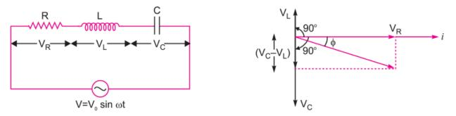
Suppose the voltage across resistance R is V<sub>R</sub> voltage across inductance L is V<sub>L</sub> and voltage across capacitance C is VC. The voltage VR and current i are in the same phase, the voltage V<sub>L</sub> will lead the current by angle 90° while the voltage VC will lag behind the current by angle 90° (fig. b). Clearly VC and VL are in opposite directions, therefore their resultant potential difference =  $V_C - V_L$  (if  $V_C > V_L$ )
