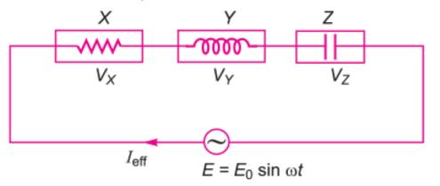
Let  $I_{eff}$  be the current flows through each element X, Y and Z. The voltage V<sub>X</sub>, V<sub>Y</sub> and V<sub>Z</sub> drop across the elements. However,
