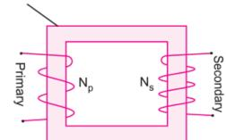
(b)Two coils on separate limbs of the core
