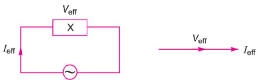
Since the phase angle between the current.  $I_{eff}$  and voltage drop  $V_{eff}$  is zero. Hence, the element X is a resistor.
