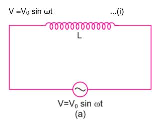
If i is the instantaneous current in the circuit and  $\frac{di}{dt}$  the rate of change of current in the circuit at that instant, then instantaneous induced emf
