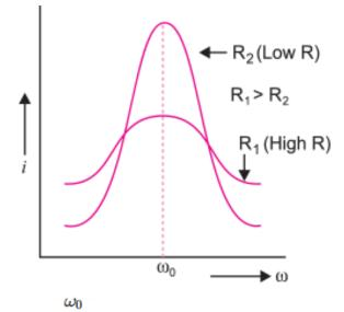
(iv)  $\overline{2\Delta\omega}$  is measure of sharpness of resonance, where  $\omega_0$  is the resonant frequency and  $2\Delta\omega$  is the bandwidth.
