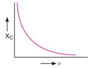
Q. 2. What will be the effect on inductive reactance XL and capacitive reactance XC if frequency of ac source is increased?
