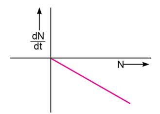
**Ans.** We know that  $-\frac{dN}{dt} = \lambda N$  where  $\lambda$  is constant for a given radioactive material. So, the graph between  $\frac{dN}{dt}$  and N is a straight line.
