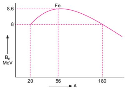
**Ans.** The graph of the binding energy per nucleon versus mass number A is shown in figure. The decrease of the binding energy per nucleon for nuclei with high mass number is due to increased coulomb repulsion between protons inside the nucleus.
