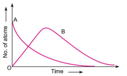
**Ans.** At t = 0,  $N_A = N_0$  while  $N_B = 0$ . As time increases,  $N_A$  falls off exponentially, the number of atoms of B increases, becomes maximum and finally decays to zero at  $\infty$  (following exponential decay law).
