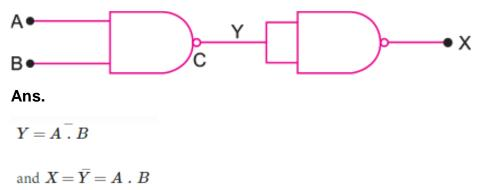
This is AND operation. Therefore, the output is 1 when both inputs are 1.
