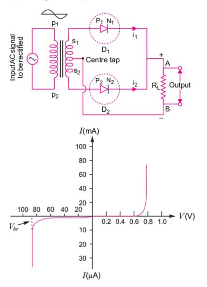
In a full wave rectifier, if input frequency is f hertz, then output frequency will be 2f hertz because for each cycle of input, two positive half cycles of output are obtained.
