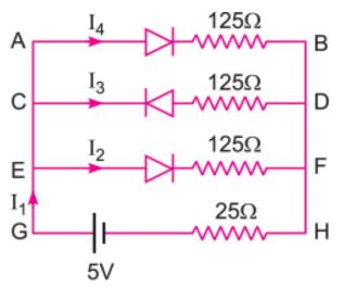
**Ans.** I<sub>3</sub> is zero as the diode in that branch is reverse biased. Resistance in the branch AB and EF are each  $(125 + 25)\Omega = 150 \Omega$
