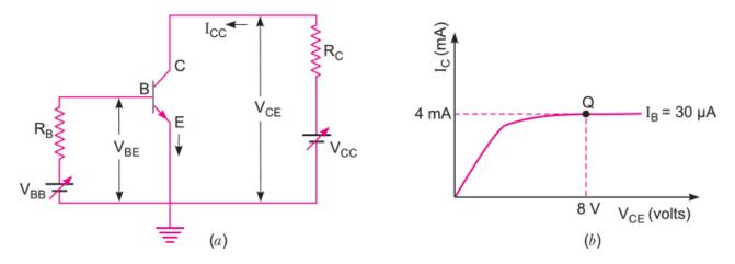
Select the values of  $R_B$  and  $R_C$  for a transistor whose  $V_{BE} = 0.7$  V, so that the transistor is operating at point Q as shown in the characteristics shown in Fig. (b).
