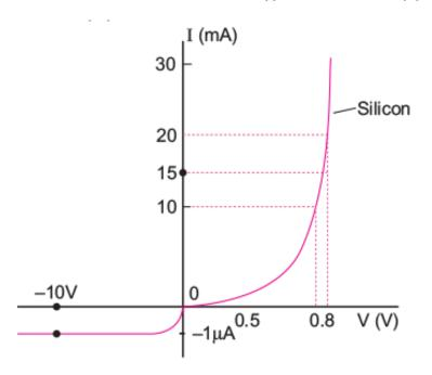
**Ans. (i)** By considering straight line of V-I characteristic curve between 10 mA to 20 mA; and assuming passing through the origin, draw horizontal and vertical lines from 10 mA and 20 mA, we have
