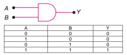
(ii) Output will be high if both inputs A and B are high., so B is in higher state in higher state in intervals from 3 to 5 and from 7 to 8.
