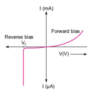
We know that reverse current is due to the flow of electrons (minority carriers) from  $p \rightarrow n$  and holes from  $n \rightarrow p$ . As the reverse bias voltage is increased, the electric field at the junction becomes significant. When the reverse bias voltage V = Vz, then the electric field strength is high enough to pull valence electrons from the host atoms on the *p*-side which are accelerated to *n*-side. These electrons causes high current at breakdown.
