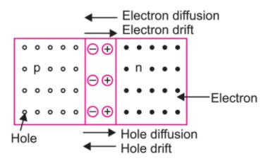
(ii) Drift: The drift of charge carriers occurs due to electric field. Due to built in potential barrier, an electric field directed from n-region to p-region is developed across the junction. This field causes motion of electrons on p-side of the junction to n-side and
