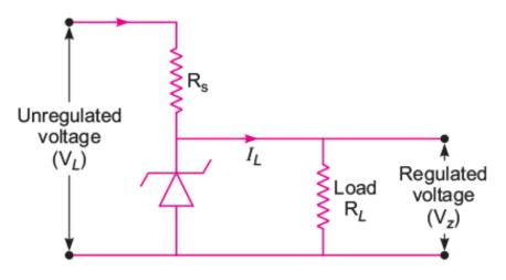
If reverse bias voltage V reaches the breakdown voltage  $V_Z$  of zener diode, there is a large change in the current. After that (just above  $V_Z$  there is a large change in the current by almost insignificant change in reverse bias voltage. This means diode voltage remains constant.
