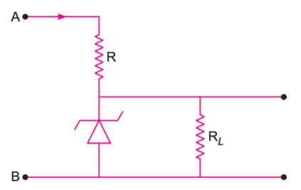
**For example:** If unregulated voltage is supplied at terminals A and B, and input voltage increases, the current through resistor  $R_Z$  and diode also increases. This current increases the voltage across  $R_Z$  without any change in the voltage across diode. Thus, we have a regulated voltage across load resistor  $R_L$ .
