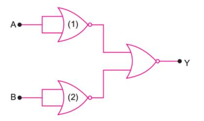
Analyse the action of the gates (1) and (2) and identify the logic gate of the complete circuit so obtained. Give its symbol and truth table.
