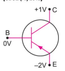
**Ans.** The given transistor is *p*-*n*-*p* transistor. The emitter is reverse biased and the collector is forward biased.
