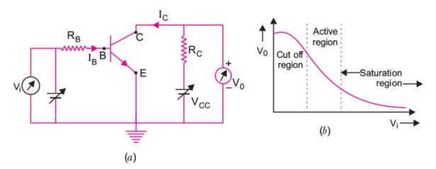
For plotting the curve the input voltage ( $V_i$ ) is changed in small steps and the corresponding output voltage is measured. The curve obtained is shown in fig. Curve is nearly linear.
