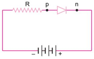
Q. 27. In the given diagram, is the diode D forward or reverse biased?
