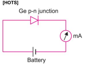
**Ans.** The internal potential barrier of germanium is 0.3 V, therefore to overcome this barrier the potential of battery should be equal to or more than 0.3 V.
