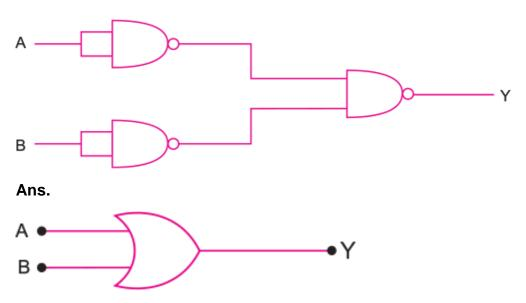
The logic circuit performs OR-operation.
