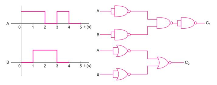
**Ans.** The output signals  $C_1$  and  $C_2$  are as shown.
