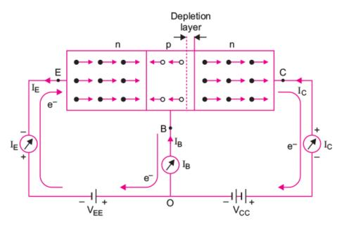
**Transistor Action:** Transistor works only when its emitter-base junction is forward biased and collector-emitter junction is reversed biased. Due to this the majority charge carriers from the emitter, accelerate to collector side and create  $I_E$ ,  $I_B$  and  $I_C$  such that  $I_E = I_B + I_C$ .
