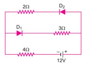
**Ans. (i)** Diode  $D_1$  is reverse biased, so it offers an infinite resistance. So no current flows in the branch of diode  $D_1$ .
