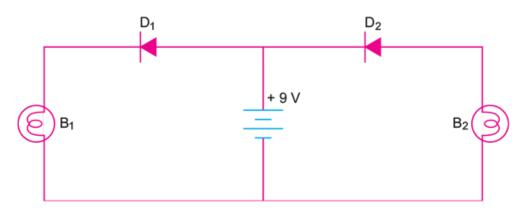
**Ans.** Bulb  $B_1$  will glow as diode  $D_1$  is forward biased.
