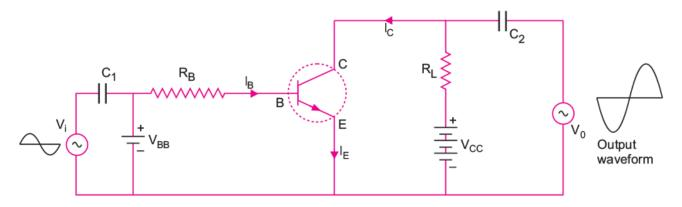
When an ac input signal  $V_i$  (to be amplified) is superimposed on the bias  $V_{BB}$ , the output, which is measured between collector and ground, increases.
