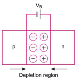
**Ans. Potential barrier:** During the formation of a p-n junction the electrons diffuse from n-region to p-region and holes diffuse from p-region to n-region. This forms recombination of charge carriers. In this process immobile positive ions are collected at a junction toward n-region and negative ions at a junction toward p-region. This causes a potential difference across the unbiased junction. This is called potential barrier.
