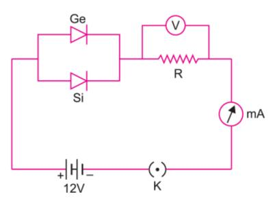
**Ans.** The potential barrier of germanium junction diode is 0.3 V and of silicon is 0.7 V. Both germanium and silicon are forward biased. Therefore, for conduction the minimum potential difference across junction diode is 0.3 V.
