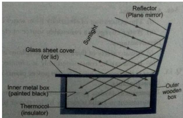
**(i) Box (B):** This is an insulated metal or a wooden box. It is painted black from inside because black surface absorbs more heat. The box may be provided with four roll-wheels.
