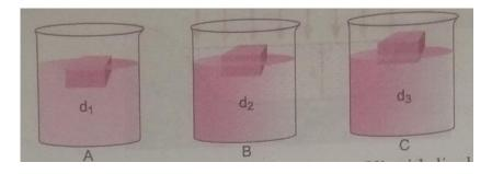
**Ans.** Liquid C has the highest density. This is because volume of liquid displaced is least in liquid C of density  $d_3$ .
