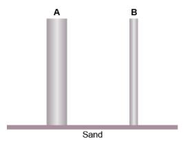
**Ans.** Rod B will go deeper as it has a smaller area of contact, therefore the same force (weight of the rod) produces more pressure. In case of rod A the same force produces less pressure.
