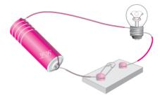
**Ans.** No. The bulb will not glow in this circuit because the switch is open and the circuit is incomplete. Due to this there will be no current flow.
