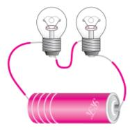
She found that filament of bulb B is broken. Will the bulb A glow in this circuit? Give reason.
