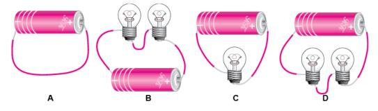
**Ans.** Arrangement A is not desirable and should not be set up. This will exhaust the cell very quickly.
