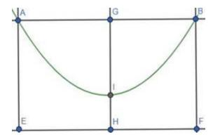
A and B are the top of the towers. AE and BF are the height of the towers. H is the center of the bridge. HI is the 5 m above from the roadway.
