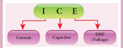
ICE is an acronym which means that the current leads the EMF (voltage) current in a capacitive circuit.
