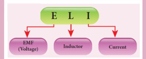
ELI is an acronym which means that EMF (voltage) leads the current in an inductive circuit.
