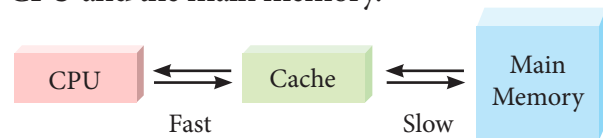
Figure 3.8 Cache Memory Arrangement
